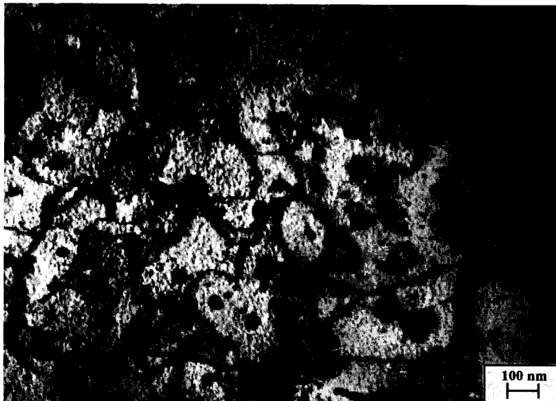
Fig. 7. Transmission electron micrograph showing the typical microstructure of dislocations and dislocation loops at the fuel center.
