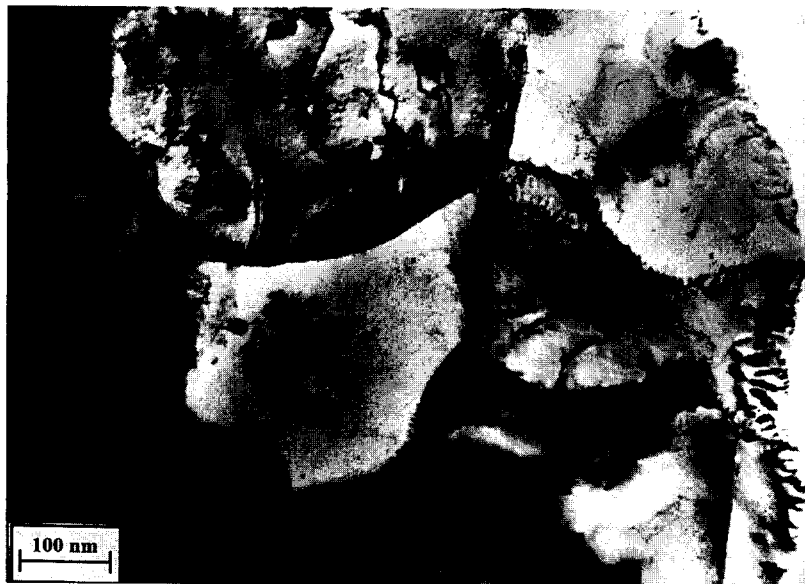
Fig. 2. Transmission electron micrograph showing the subgrain structure at the rim of the fuel, demonstrating the low density of dislocations found within the structure. A low density of precipitates is found, but fission gas bubbles are almost absent.
