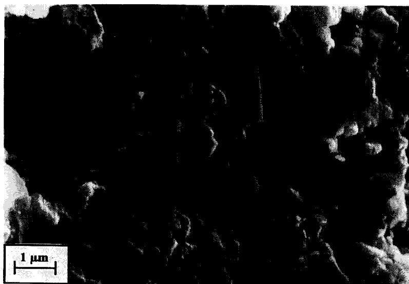
Fig. 10. Scanning electron micrograph of the typical subgrain structure found at a depth of 1200 \mu\text{m} from the fuel surface.
